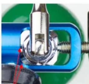
Proper washer seal and fit. Regulator yoke is flush to valve
