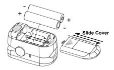
Please put in the batteries according to the polarity marked inside the battery compartment.
