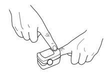
There are 4 display modes. After turning on the pulse oximeter, each time you press the power switch, the pulse oximeter will switch to another display mode.
