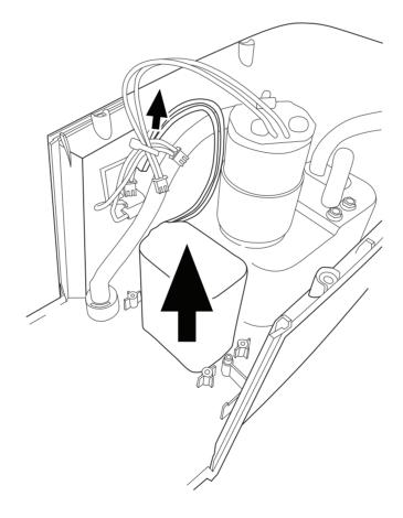
The new battery will also include replacement wires. Install new battery and wires in place of old battery.
