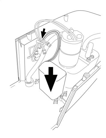
Replace the white battery case with 3 screws as shown.
