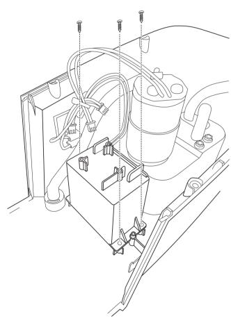
Remove the old blue battery including its attached wires.
