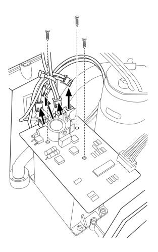
Remove the 3 screws from the battery case as shown, then remove battery case.
