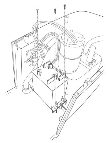
Replace the circuit board with 3 screws and plug the wires back in as shown.
