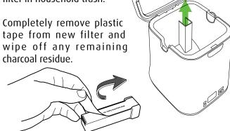
Place new filter into holster and press down until it is fully seated.
